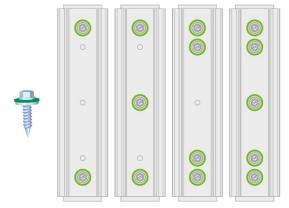
The static calculation in the system planning defines the number of fasteners required for mounting modules in landscape.
