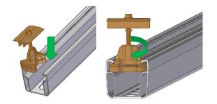
Insert the middle clamps or end clamps at the clamping position from above into the rail chamber. Then turn the rail nut in the rail and push the module clamps towards the module frame.
