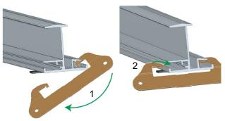
Place the insertion rail onto the EPDM strips, maintain 10 mm gap at the rail joint, Hook the trapezoidal sheet bracket into the rail on one side, feed it below the rail (1) and hook it in on the other side (2). The trapezoidal sheet brackets must be hooked into the insertion rail on both sides.
