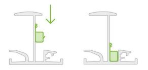
A contact latch must be fitted under each module. The contact plate must be pressed into the channel onto the bottom of the insertion rail.
