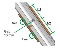
The number of fasteners is based on the static calculation with the fasteners shown.
