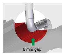
Height adjustment of the roof hooks through the thread in the base profile. The distance between the bottom tile and bracket must be 6 mm after attachment.
