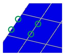
The modules must then be attached to the rails using end clamps and middle clamps.
