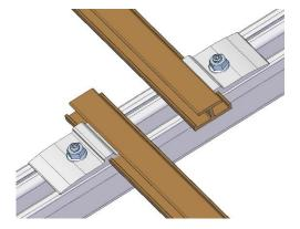
Dependent on the module load it might be necessary to install a support rail centred under the module. Attachment is with the Cross rail connector set C IR M8. The support rails must be fitted parallel to the insertion rails and must be offset on the C-rail in the overlap area.
