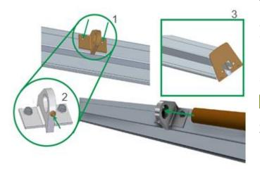
The mounting brackets snowguard IR have to be fixed on the insertion rail Plus with two drilling screws (1). Position the round pipes centrally and fix them with the grub screw (2).
