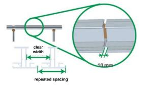
Fasten insertion rail Plus on C-rails with cross rail connector set C ES like insertion rail. Insert connector insertion rail Plus up to the stop and push the second rail over the rail connector with a distance of 10 mm.
