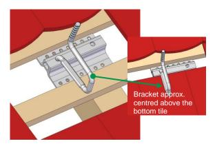
Install the roof hook with the long side of the base profile facing down. Position the bracket whilst maintaining the lateral overhang (MV 1.4) approx. centred above the tile below.
