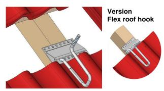
Insert roof hook with the bracket positioned in the trough of the roof tile. The position of the roof hook on the rafter must be defined taking into account the static specifications (MV 1.4). Mark the top tile and, if necessary, the bottom tile at the roof hook exit point. For plain tile covering proceed according to MV 1.2 + 1.3.
