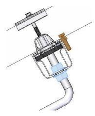
Prior to mounting the modules the slip guards must be fitted to the frame holes above the bottom rail position (MV 4).
