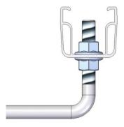
Place the C-rail onto the lower self-locking nut, align the rail and tighten it with the top self-locking nut. The roof hook can also be connected to the rail connector in the joint area. For mounting in the cross rail arrangement (insertion/clamping system) the top rail is attached using the cross rail connector or Cross rail connector set C IR M8 (MV 2).
