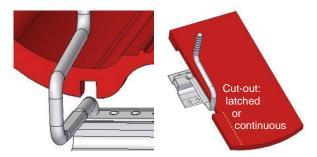
Interlocking tiles / concrete roof tile: At the exit area of the roof hooks carefully make a cut-out with the angle grinder.
