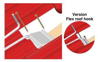
Attach the roof hooks to the rafter with wood screws (MV 1.4). The screw length depends on the roof design and is determined by the calculation software. If the counter battens were not taken into account in the design software or mounting is on a rafter insulation, the base profile of the roof hook must be padded on both sides of the counter batten for at least the width of the rafter.
