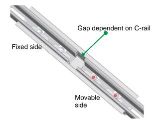
MV 3.3 Mounting expansion joints for C-rails
