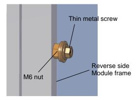
Push the nut over the screw and screw the thin metal screw into the module frame without predrilling.
