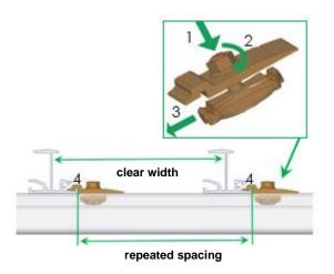
Insert the Cross rail connector set C IR M8 into the rail groove (1) from the top, rotate the nut by 90° (2) and push the component against the insertion rail (3) until the Cross rail connector set C IR M8 engages with the mounting flange (4).
