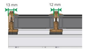
End clamp mounting flush with the rail end possible.
