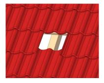
Expose the rafters by removing the tiles.
