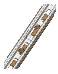
Join the rail ends flush, apply the rail connector centred and connect it to the rail using the mounting screws included in the set. The connector and number of screws depend on the rail (MV 3). Maximum uninterrupted rail length 13 m, then install expansion joint or disconnect the rail (MV 3.3).
