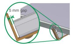
Screw the slip guard to the rail end with approx. 5 mm gap using mounting screw and self-locking nut.
