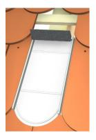
Determine the position of the sheet metal tile. Replace tile with plain tile sheet – the metal sheet edges are below the adjacent tiles – and secure with screws, then glue on foam wedge.
