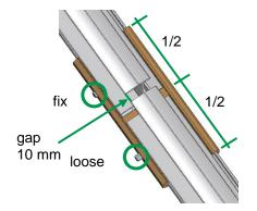
Push the rail connector over the mounted rail in the middle and tighten the first grub screw. Push the rail to be connected into the connector, gap between the rails 10 mm, tighten second grub screw without play.
