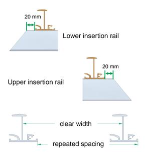
The distance between the lower and upper insertion rail to the edge of the support surface to the end of the module field at the bottom and top is 20 mm.
