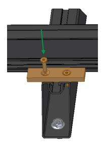
Mount the slip guard device under the lowest insertion rail on each socket with two drilling screws, starting with the right-hand screw, centrally and without gaps.
