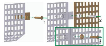
Push the connector for the perforated sheet approximately centrally under the already mounted perforated sheet and fasten it with the drilling screw and countersunk washer through an opening (1). Place the subsequent perforated plate flush and fasten it using the same principle (2). If necessary, the perforated plates must be cut to the required length with a sheet metal scissors.
