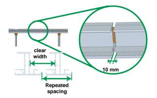
Attach the Insertion Rail Plus to the C-rails with mounting set insertion rail M8 as the insertion rail. Insert the connector for Insertion rail Plus up to the stop and push the second rail with a distance of 10 mm over the rail connector.
