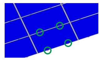
The modules must then be attached to the rails using end clamps and middle clamps.
