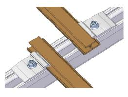
Attach the support rail IR with the Cross rail connector set C IR M8 - the support rails must be fitted parallel to the insertion rails and must be offset on the C-rail in the overlap area.
