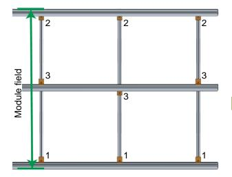
For the top and bottom insertion rail of the module field the mounting set insertion rail M8 is fitted on the inside in each case (1, 2). At the centre insertion rails the mounting set insertion rail M8 must be fitted alternating at the top and bottom at the mounting flange (3).
