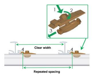
Insert the Cross rail connector set C IR M8 into the rail groove (1) from above. Rotate the nut by 90° (2) and push the component against the insertion rail (3) until the Cross rail connector set C IR M8 engages with the mounting flange (4).
