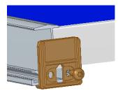
Centre the rail connector over the fitted rail and tighten the first threaded pin. Push the rail to be connected into the connector. Gap between rails 10 mm, tighten the second threaded pin without play. MV 7 must be complied with for the mounting of the Insertion Rail Plus rails.
