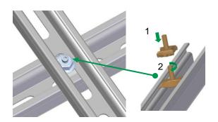
Place rail ends onto the gap, apply the rail connector and connect it to the rail at the fixed and movable sides using the mounting screws. Tighten the screws firmly on the fixed side. The screws on the movable side are coated in red and must be released again after tightening (approx. ½ turn). Maximum rail length with expansion joint 40 m, then plan proper rail disconnection.
