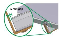
Prior to mounting the module screw the slip guard to the rail end with approx. 5 mm gap using mounting screw and self-locking nut (MV 6.1/6.2).
