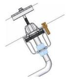
Prior to mounting the modules the slip guards must be fitted to the frame holes above the bottom rail position.
