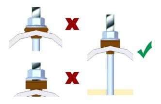
Tighten the lower self-locking nut until the EPDM seal is slightly compressed – the seal cone enters the predrilled hole of the roof cover.
