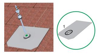
Position the projection of the metal shingle above the drill hole and screw in the stock screw.
