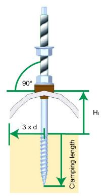
Draw the axis of the mounting rails on the corrugated crests / raised beads. Mark the position of the stock screws along the rail axes above the purlins.
