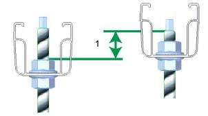
Place the C-rail onto the lower self-locking nut, adjust the rail height by appropriate positioning of the self-locking nut (1). Then tighten the upper selflocking nut.
