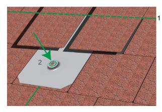
If necessary detach the shingle above, push the metal shingle flush up to the top edge of the roof shingle row below (1) and align. Then mark the position of the stock screw (2) through the hole (d = 14 mm) in the metal shingle and predrill the rafters through the roof cover in accordance with the stock screw size (MV 1).
