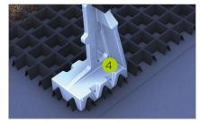
Positive fit of substrate plate and support
