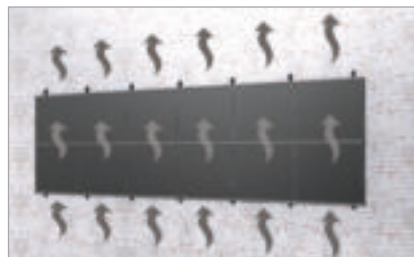
Very good rear ventilation of the modules
