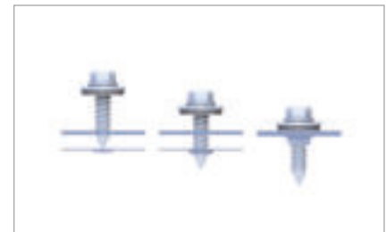
Chipless screwing for high holding forces
