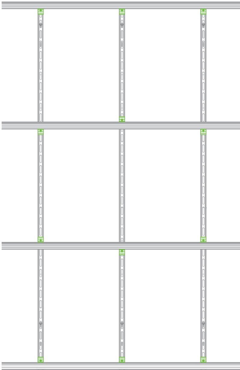
**B** Positioning cross-rail connector set IR.
