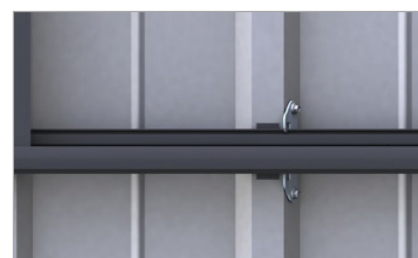
Fastening the trapezoidal bracket to the high bead
