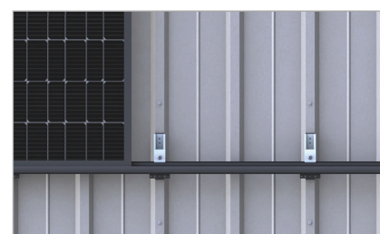
Fixing of short profiles to the facade
