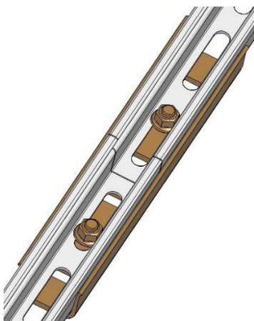
Join the rail ends flush. Apply the rail connector centred and connect it to the rail using the fastening screws included in the set. The connector and number of screws depend on the rail (MV 3).
